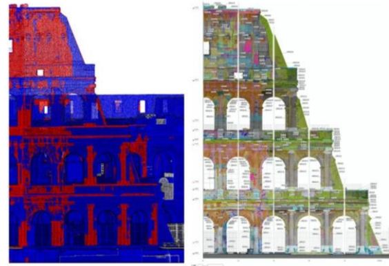
Figure 14: Left: decay mapping on the 3D point cloud, in red the surface runoff; right: decay mapping on the 2D drawing highlighting decay overlappings.
